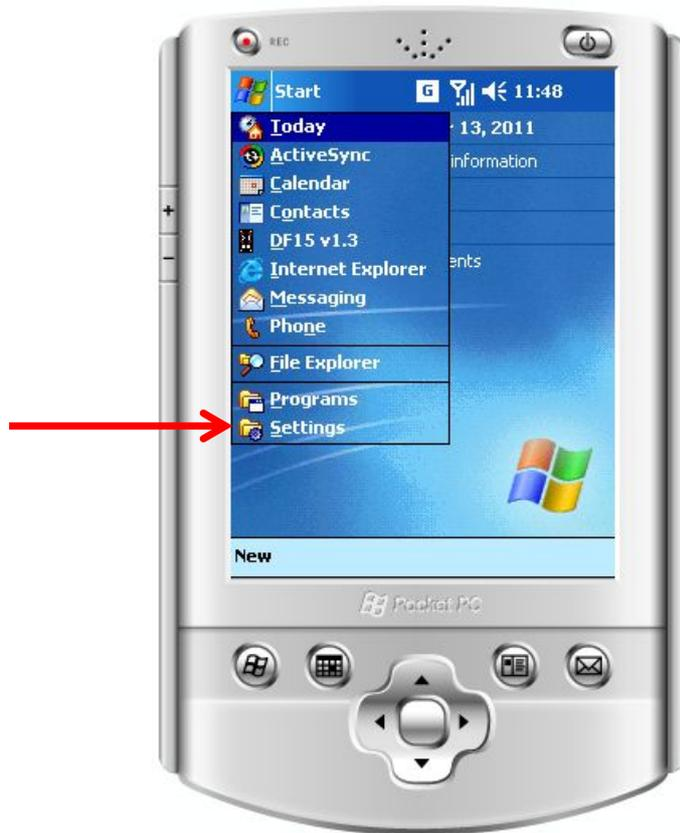
Then after selecting the System Tab at the bottom of the screen click on Clock and Alarms
