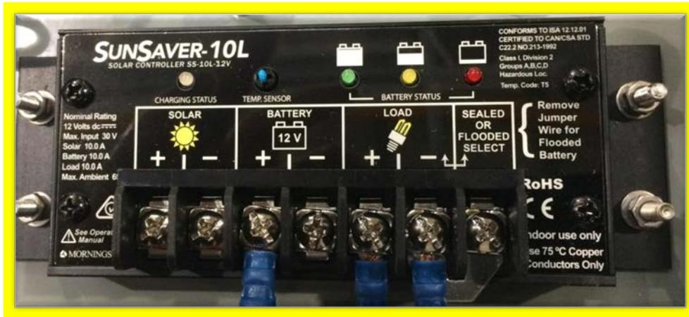
The Red 'Load Disconnect' LED will light to indicate that the charge controller has automatically disconnected the DF15 where the battery charge is very low in order to prevent potential damage. The controller will automatically turn the DF15 back on once the battery charge has returned to acceptable levels Solar Power connection is now complete and the DF15 is ready for sign configuration parameters to be set and deployment. (See section 3)
