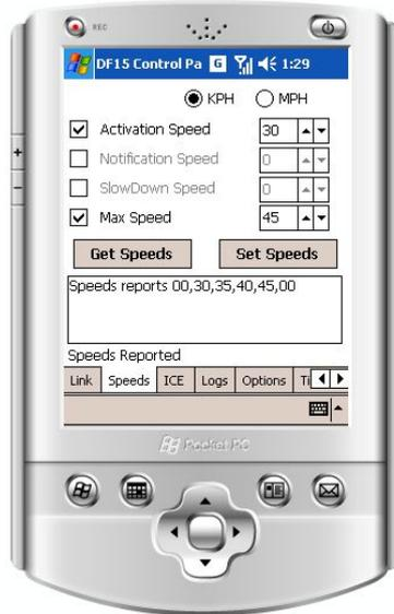
This following combination would cause the sign to go straight to a speed feedback display plus flashing Beacons at 45. (where the Beacons are disabled the display would flash) At 50 the display would alternate between the speed display and the SLOW DOWN legend; and at 55 the display would change to the SLOW DOWN legend only with flashing Beacons where selected.
