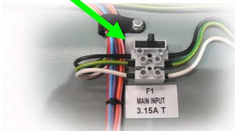
This fuse protects the equipment against AC supply voltage anomalies and is a time delay fuse rated at 3.15 Amps
