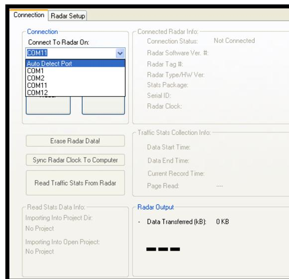
If you select Auto Detect the system will try each port individually to detect the Bluetooth™ Device and this could take some time to achieve. As soon the system has connected with the radar a dialogue box will confirm the system setting information and then a Radar Found Pop Up will appear. You can clear these boxes by clicking OK. (You may wish to note the COM Port used to speed up future connection processes):
