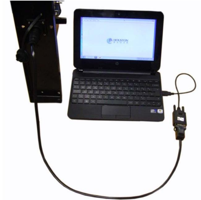
The DF11 features a standard cable interface that can be used to configure the display and download captured speed data onto a Laptop/PC running the Stats Analyzer software. The cable plugs directly into the multi-function socket located on the base of the unit. The cable only needs to be finger tight and any excess force applied will result in damage to the connectors, which may not be covered by any warranty.
