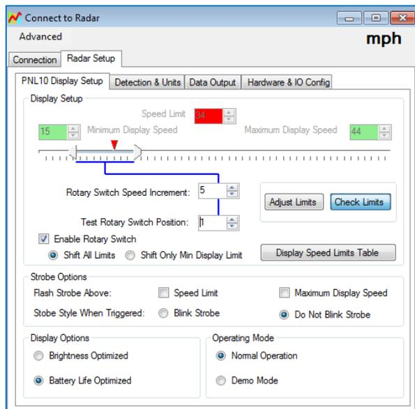
Clicking the 'Display Speed Limits Table' button will bring up a handy table showing the parameters each rotary switch position is set to. This can be printed and kept with the sign if required.
