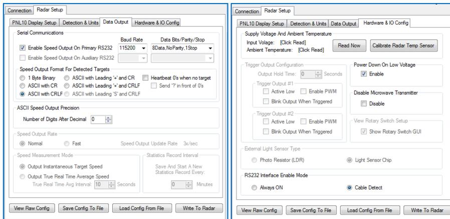
The settings in these tabs are factory set. If any of the values are altered without first consulting Unipart Dorman, the performance of the sign may be severely degraded and could result in the sign being returned to works for resetting, which would be outside any warranty agreements.
