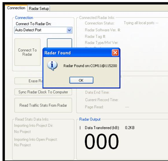
The Radar Found box will display a data transfer speed, it should be noted that these speeds are variable depending on a number of different things. However, if you feel the data transfer speed is excessively slow, please contact Unipart Dorman for advice.
