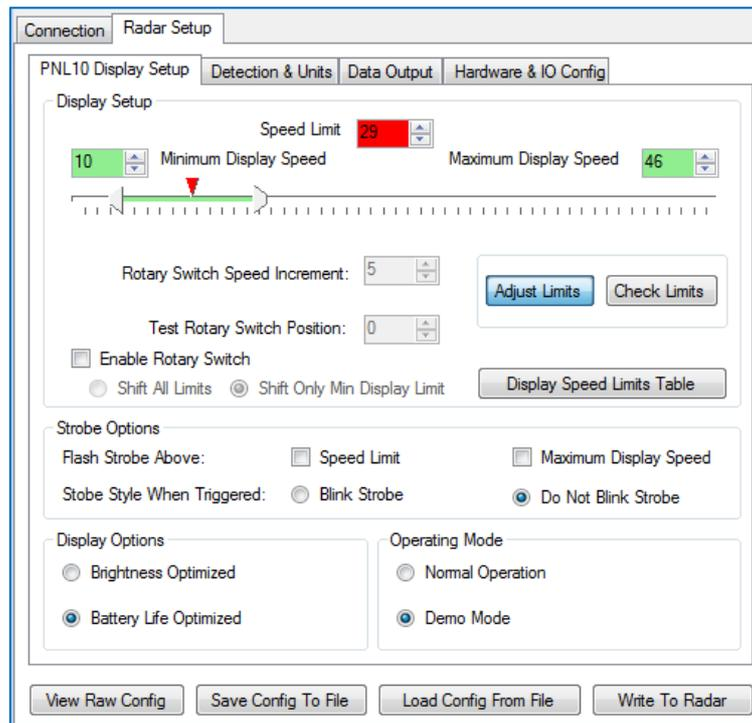
The Minimum setting should be set sufficiently high to prevent the sign being triggered by for example a jogger approaching the sign, but low enough to capture approaching motor vehicles. Careful consideration of this value will allow the sign to create the maximum impact but preserve battery life as much as possible.
