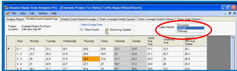
The Monthly Counts/Speed Avgs tab shows in a weekly view the average counts or speeds for a specific hour segment averaged over an entire month. The values highlighted in Orange show the highest speed for the timeframe selected. Available months are shown and selected in the drop down circled in red on the picture above.
