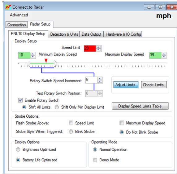
The 'Check Limits' selection allows the user to cycle through the parameters already set into the sign.
