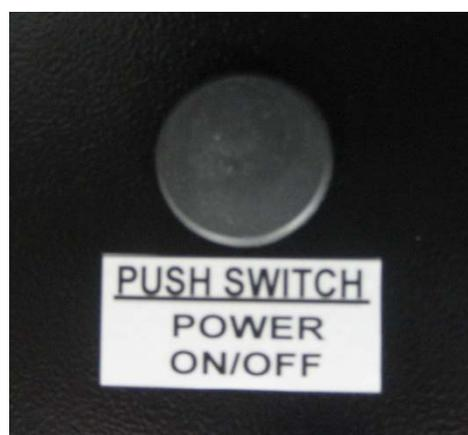
It should be noted that the switch is covered by the adaptor plate when the sign is fitted to it. This security feature prevents malicious operation.
